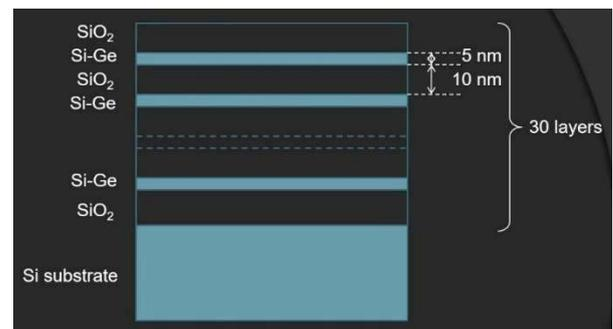
**Fig. 3.** the schematic diagram of the multilayer structures of  $\text{Si}_{1-x}\text{Ge}_x$  and  $\text{SiO}_2$  were prepared by co-sputtering method on quartz substrates or Si substrates
